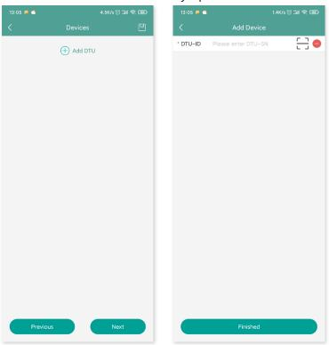
6. Scan or manually input the microinverter ID. Press "Finish" when all microinverter IDs have been input.
