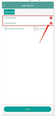
5. Confirm that the microinverter ID in the list is correct, and tap save.
