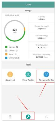
✓ Select the DTU's wireless network and click "Connect". (The network name of the DTU consists of DTUP and product serial number. In the following example, the DTU ID is 65200316 and the network name is DTUP-65200316.)
