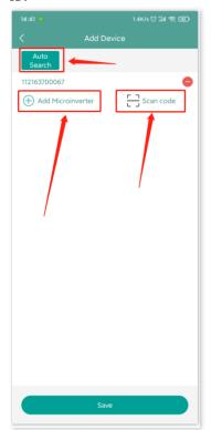
4. The search result of microinverters and microinverter added will be displayed in the list. Tap the button on the right if you want to delete it.
