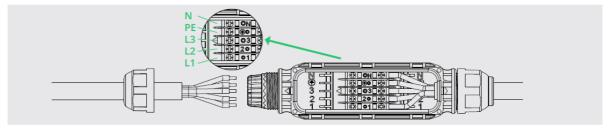
• Tighten the screws and tighten the cap back to the port.
