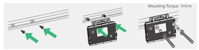
3. Hang the microinverter (label side up) on the screws and beneath the PV module. Then tighten the screws.
